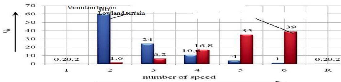
Fig.3. Gearbox speed ratio when driving on mountain and lowland terrain
