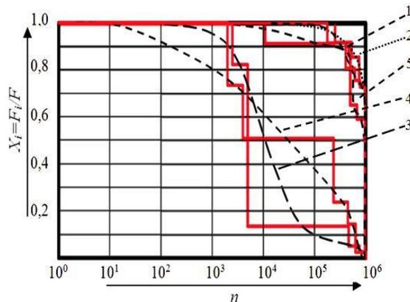
Fig.7. Load spectrum for all bearings in the six-speed gearbox
