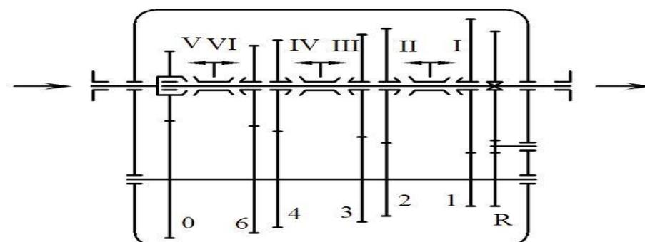
Fig.1. Bearings and gears position in the gearbox
