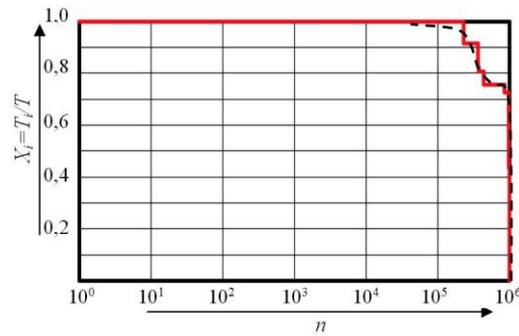
Fig.6. Load spectrum for the bearing on the input shaft
