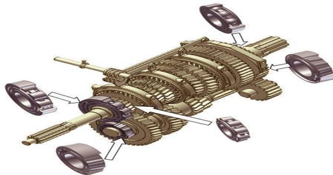
Fig.2. Six-speed gearbox with a 3D display of the interior of the gearbox
